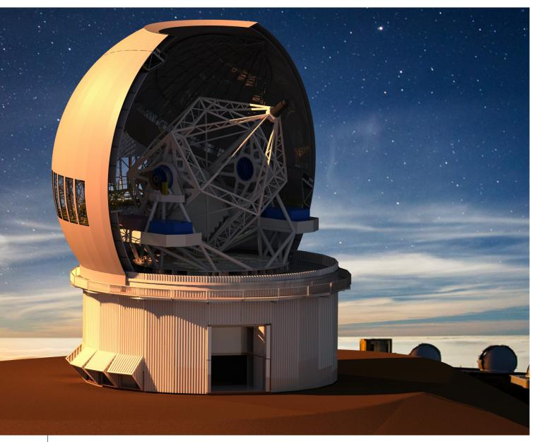
CFHT is using SOLIDWORKS software to support implementation of the Maunakea Spectroscopic Explorer, a 10-meter-class telescope that is fully devoted to spectroscopic exploration of the universe and the only facility of its kind.
